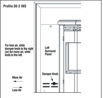
Figure 11 - Damper Adjustment, Inserts
